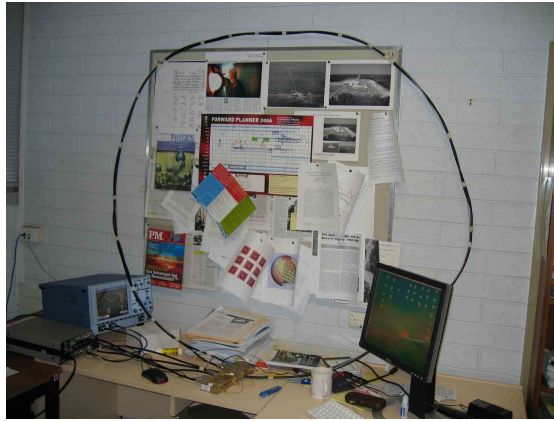
Figure 13: The Flinders University Gravitational Wave Detector showing the cables formed into a loop. This configuration enables the calibration of the detector. The data from such a looping is shown in Fig. 14, but when the detector was relocated to an isolated underground laboratory.
